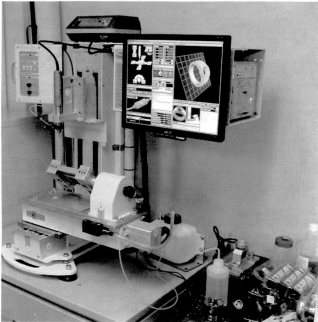
↑ Revo 540b Milling System – wax models for casting ↑
